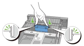
3 Load paper in the standard 250-sheet tray, and then insert the tray into the printer and push until it stops.
